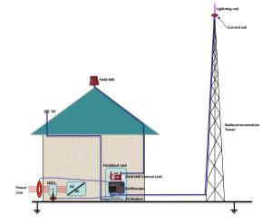
Fig. 1. Functionnal diagram of the experiment
