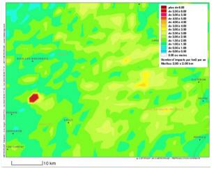
Fig. 2. Ground flash density in the experiment area
